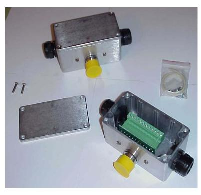
This product is intended to mount on the die shoe and allow a maximum of eight sensors to wire directly to it.
